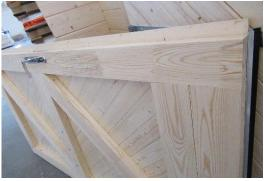
Hang door on hinges that are assembled on frame
